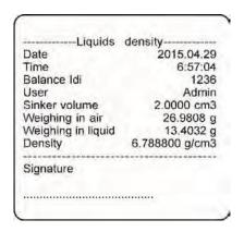
To finish density determination process, press key. The home screen for liquid density mode is displayed. The next measurement can be started now. The balance operates with previously entered settings (sinker volume) thus providing quicker start of the very measurement.
