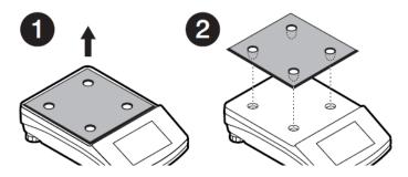
2) Check that the grounding spring is in the correct location, the spring juts slightly out of the hole.
