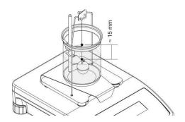
10. Upon confirmation of the second indication, the software automatically calculates measured liquid density, which is next displayed together with a respective message.
