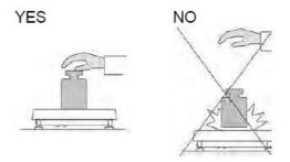
• Place weighed load in the center of the weighing pan:
