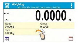
Press and hold the spot where the label is to be placed.
