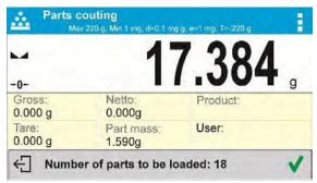
• The balance automatically recalculates single part mass, next it moves to <Parts counting> mode displaying number of parts loaded on the weighing pan (**pcs** marking).
