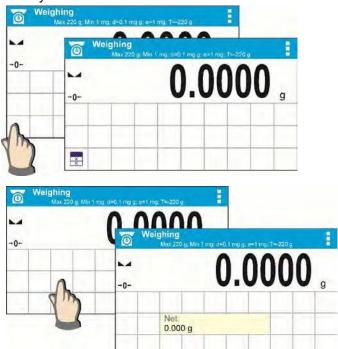
3. A new widget can only be applied to an area that holds no other widgets. The balance automatically detects which widgets can be applied to an area, this is conditioned by the widget dimensions.
