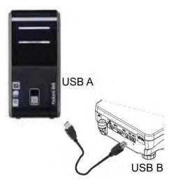
Having completed driver installation, connect balance to a computer, use USB A/B cable (in case of already connected balance, it is necessary to disconnect it and using USB cable connect the balance again).
