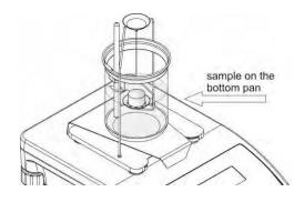
12. Upon confirmation of the second indication, the balance automatically calculates measured solid density, which is next displayed together with a respective message.
