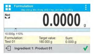
At the top of information area there is a bar graph, underneath the bar graph weight value that is to be dosed is displayed. Bar graph color changes gradually depending on the ingredient weight (read Dosing section for detailed description of bar graph).
