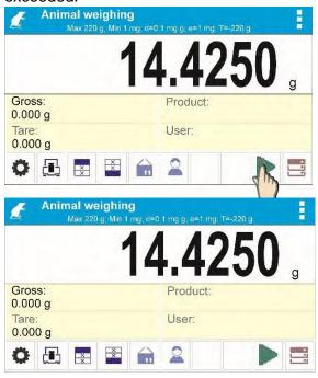
• On completed mass determination process, "freezed" weighing result is displayed, the mass is automatically printed using the printer.
