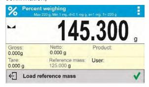
• 100.000% indication is displayed, loaded part weight is accepted as a reference mass, it is automatically recorded and displayed in reference mass field.
