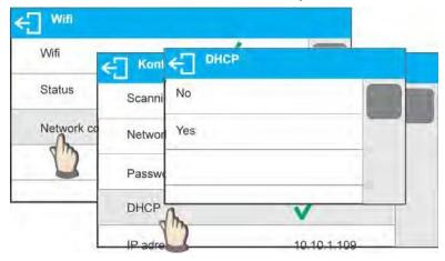
With DHCP set to NO value, enter manually IP; MASK; DEFAULT GATE parameters, with DHCP set to YES value, the balance software automatically reads and displays data assigned by Wi-Fi router by means of which the balance is to be connected  Enter <SCANNING NETWORKS> parameter and start network searching procedure, upon completion, list of detected networks is displayed along with information on signal strength and channel number
