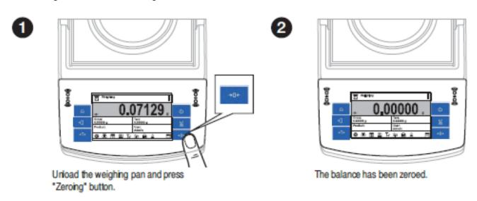
The Zeroing process is an equivalent for determining new zero point, recognized by the balance as precise zero. Zeroing is possible only for stable status of display indication.
