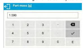
• Enter the requested value and confirm by pressing key, <Parts counting> mode is run with automatically specified part mass.
