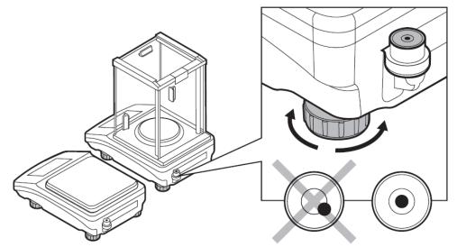
The balance should firmly rest on a surface, each of the feet must be supported.
