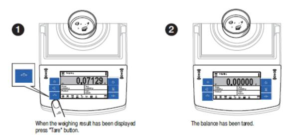
The balance enables assigning tare value to a database-stored product. Using this option, the software automatically uploads data on tare value for a product upon its selection from the database.
