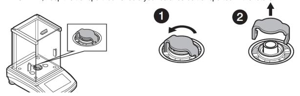
2) Check grounding spring to insure it is in the appropriate location. Make sure that the grounding spring juts slightly out of the hole.
