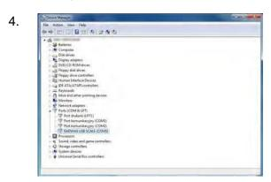
Go to Device Manager and check number assigned to virtual COM port.
