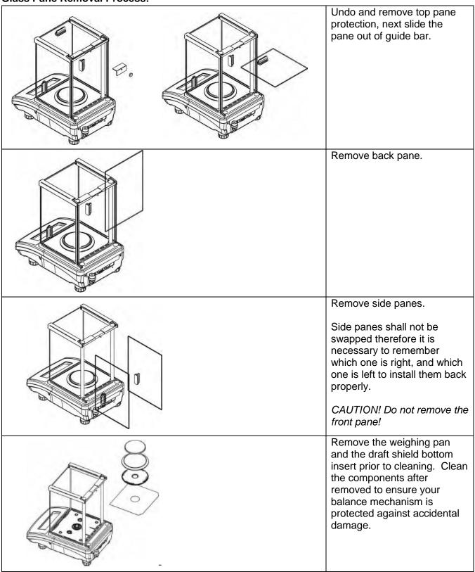
All the operations should be done carefully. Pay special ATTENTION to the spot where the weighing pan was installed: dirt and other small elements might enter the balance construction through this opening, which might negatively influence the balance parameters.
