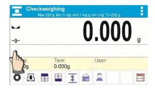
Press and hold the spot where bar graph is to be placed.
