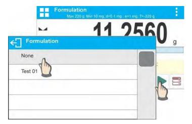
Home screen is displayed, container weight is tared automatically, navigation bar with messages for ease of operation is shown
